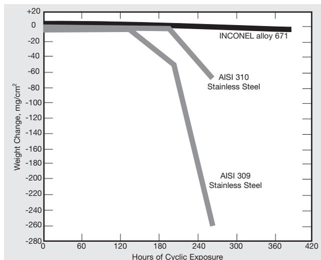
**Figure 2.** Cyclic oxidation tests at 1800°F (980°C) on specimens coated with Na<sub>2</sub>SO<sub>4</sub>. Each cycle was 15 minutes heating/5 minutes air cooling. Specimens re-coated at 65-hour intervals.
