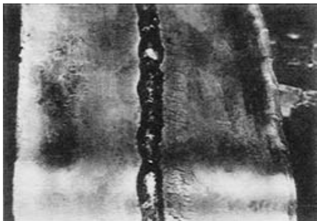
Figure 3 Nickel 200 showing sulphur embrittlement of sheet on the right side caused by inadequate cleaning. Photo courtesy Inco Alloys International Inc.
