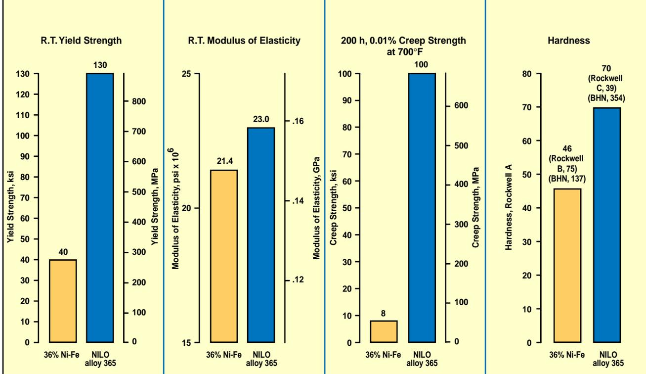
Figure 3 – Mechanical property comparisons between annealed and age-hardened NILO alloy 365 and a typical, annealed, 36% nickel-iron alloy. Note the moduli data offering the opportunity to reduce cross-sectional area in larger tools, thus a reduction in the amount of alloy used for the tool. Also, note the higher hardness for better protection against scratching by knives during the laying-up process.
