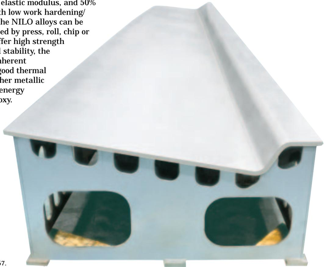
A NILO alloy 36 mandrel on a tool assembly for the Boeing 757.
