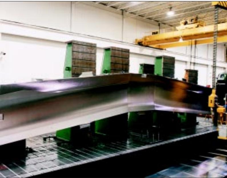
45 ft (13.7 m) bond jigs in NILO alloy 36 for the upper and lower wing skins of the Bell Helicopter V22 Osprey. (Remmele Engineering, Inc., General Machining Division, New Brighton, Minnesota, USA).
