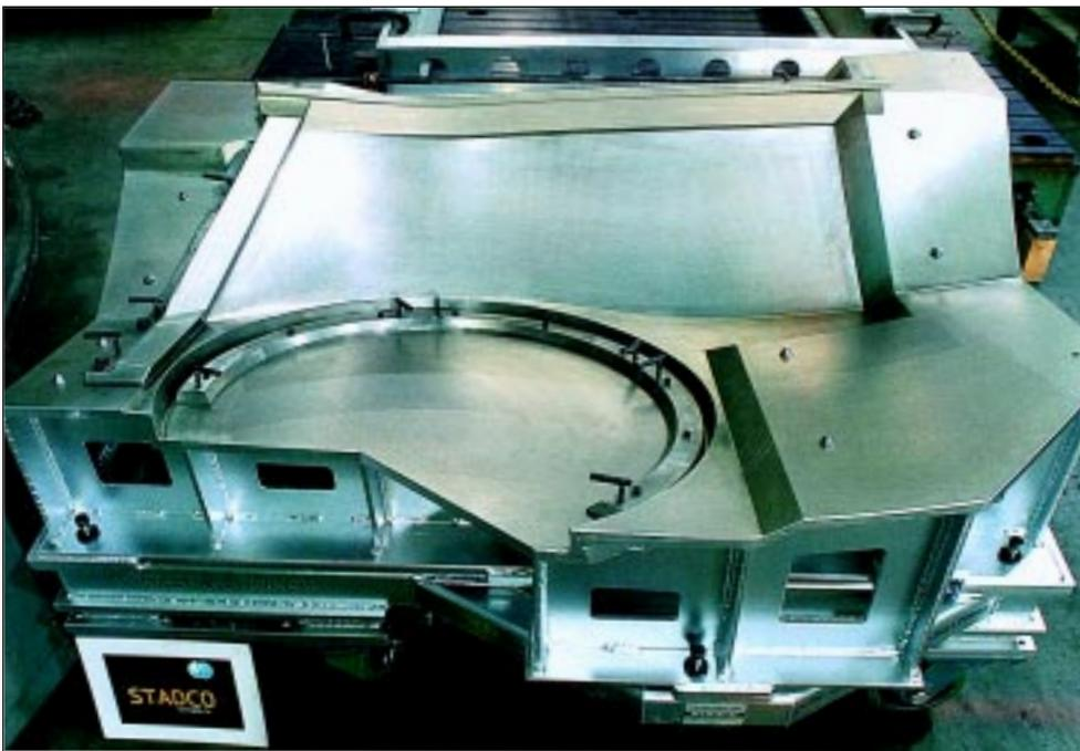
A NILO alloy 36 tool for the upper skin of the Sikorsky Comanche helicopter. This intricate mold shows removable inserts allowing undercut contours without creating lock-on conditions. (STADCO, Los Angeles, USA).
