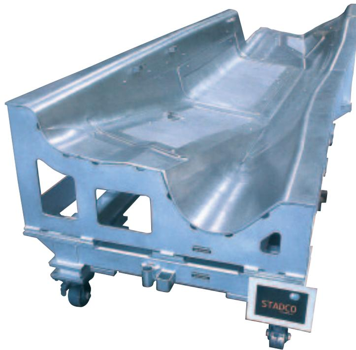
A NILO alloy 36 lay-up tool for the canopy structure of the Sikorsky *Comanche* helicopter. Inset, one of these tools is being probe tested to confirm the high-precision manufacturing tolerances. (Remmele Engineering, Inc., General Engineering Division, New Brighton, Minnesota, USA).
