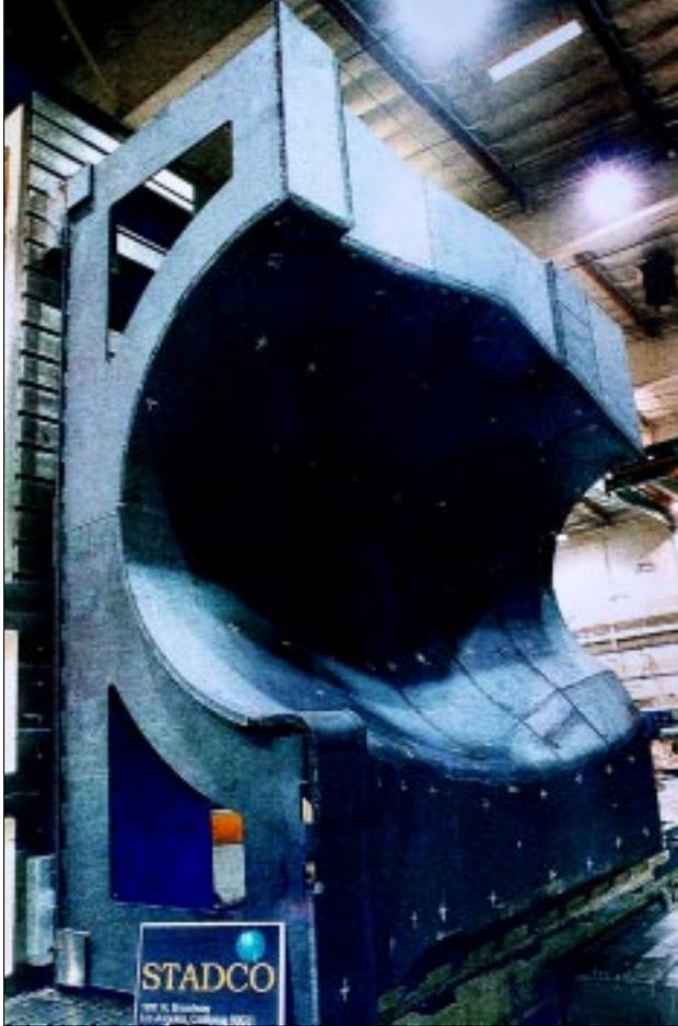
A mid-engine cowl bond jig tool in NILO alloy 42 for a Pratt & Whitney engine on *Airbus 340*. (STADCO, Los Angeles, USA).
