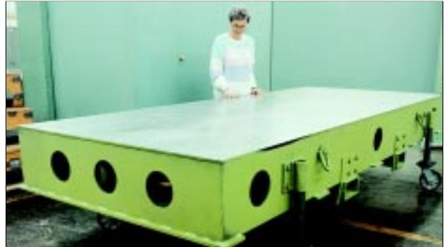
This NILO alloy 36 flat plate tool was the first full-scale prototype in service at Boeing over ten years ago. It was in use more than 500 production cycles later, the performance having exceeded steel, aluminum and graphite epoxy tools for consistency and reliability. Special Metals was told that Boeing would not give up the alloy tool for “post mortem” analysis — it was still required for production.
