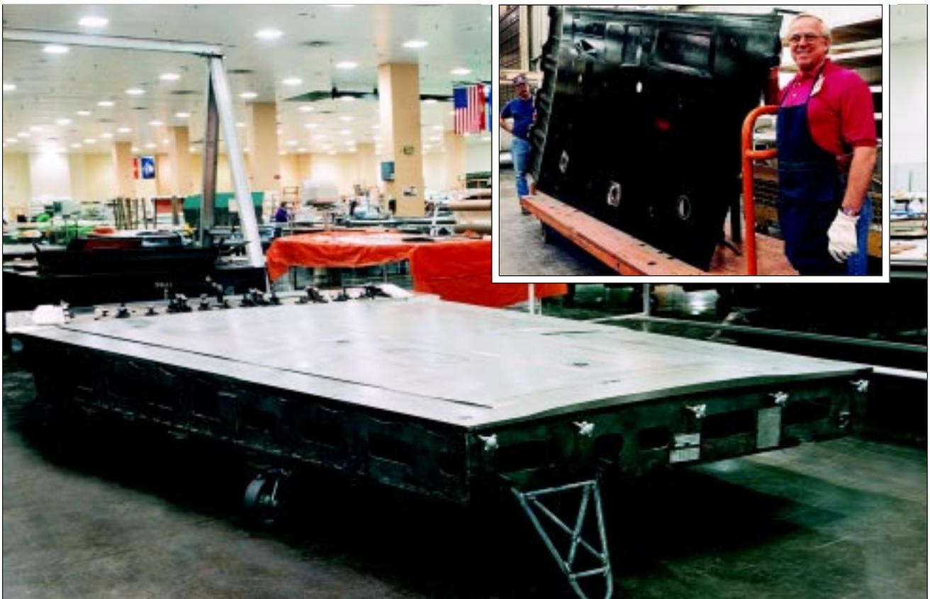
A complex NILO alloy 36 tool, 25 ft (7.6 m) long, made to  $\pm 0.005$  in (0.13 mm) tolerances. (STADCO, Los Angeles, USA).
