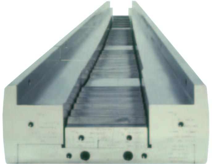
A NILO alloy 36 tool for the horizontal stabilizer of a McDonnell-Douglas F-18E/F. The inset picture shows the actual part produced with co-cured titanium root fittings.
