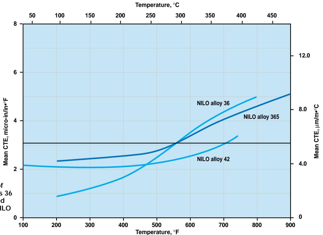
Figure 2. A CTE comparison of annealed NILO alloys 36 and 42, with annealed and age hardened NILO alloy 365.
