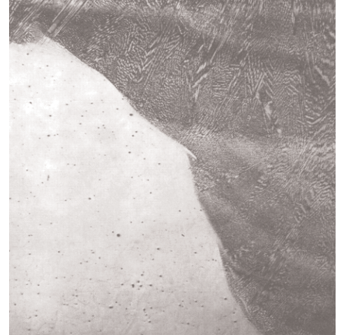
Figure 15 - Photomicrograph illustrating fusion and adjacent heat affected zone integrity of gas tungsten arc welded INCOLOY alloy 864. Etchant - Nital. Magnification: 20X
