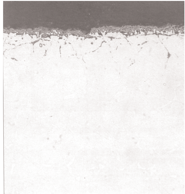
Figure 7 - Photomicrograph of the as-polished cross section of an INCOLOY alloy 864 burner rig sample after 500 h exposure at 950°C (1742°F). Magnification: 500X
